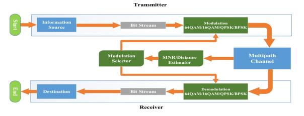
Figure 1: Block diagram of adaptive modulation system.
