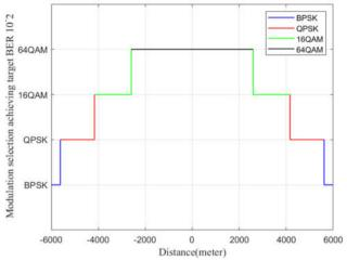
Modulation schemes selection based on Distance in AWGN Channel
