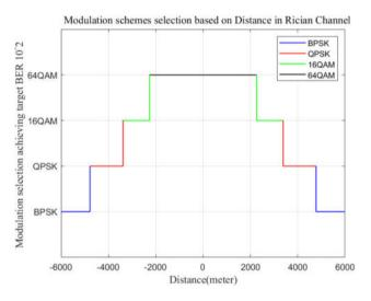
Figure 11: Illustration of distance-based selection of various modulation schemes in Rician channel.
