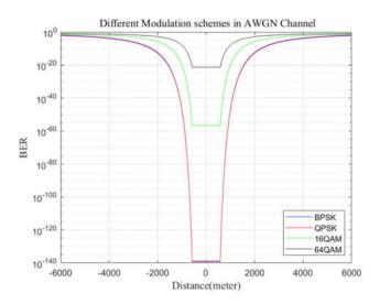
Figure 3: BER vs. distance of different modulation schemes in AWGN channel.
