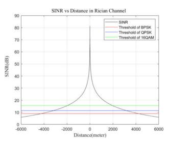
Figure 10: SINR vs. distance in Rician channel.
